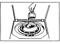
7. Add fabric softener, if desired. Place the Fabric Softener Dispenser on the Filter-Flo pan. Pour 1 teaspoon (5 ml) of concentrated softener or 1 tablespoon (15 ml) of diluted softener into a standard measuring cup. Add enough water to fill the cup 1/2 full. Pour the diluted softener into the dispenser. See page 9 for dispenser instructions.
